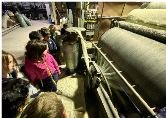
The carded wool being taken off the final drum at the end of the machine
