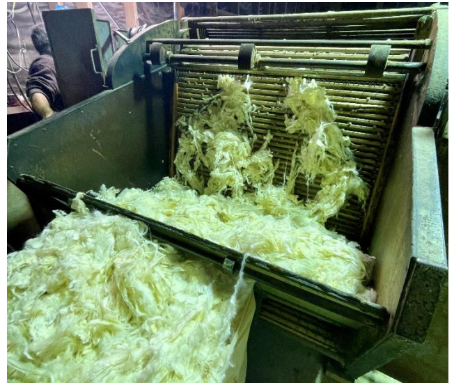
The carding machine starts up, picking up the raw fleece
