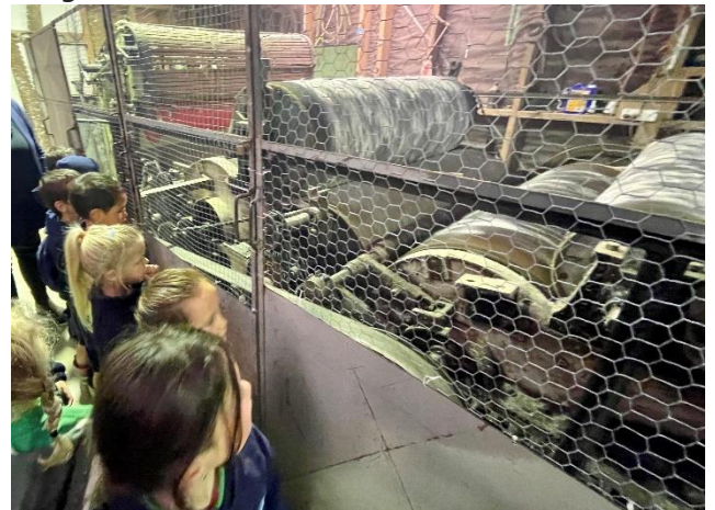
The drums spinning as they card the wool
